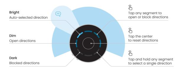
Device orientation: open segments face the group, blocked segments face you
